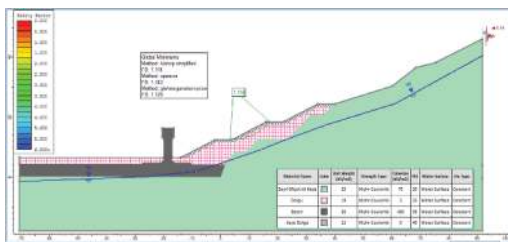
Figure 10. Seismic stability analysis of the diversion tunnel entrance conduit section (FS= 1.118 > 1.1).
