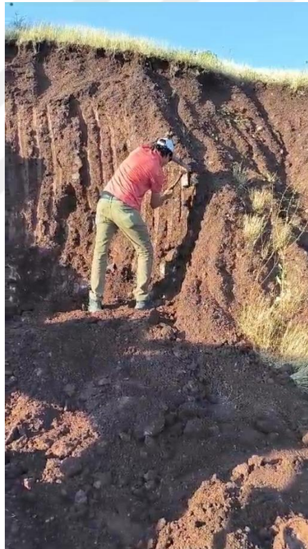
Image 3.1. In-situ extraction of undisturbed samples from the exposed slope face
