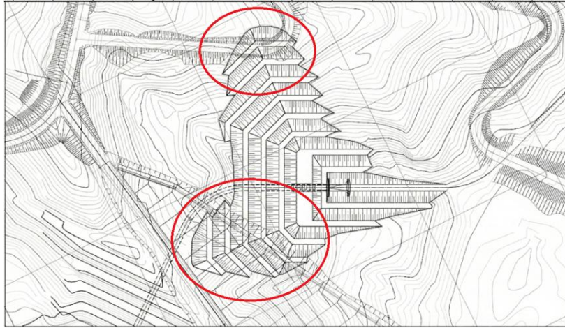
Figure 4.53. Schematic plan illustrating the the infeasible permanent 1V:1.5H slope at the diversion tunnel inlet
