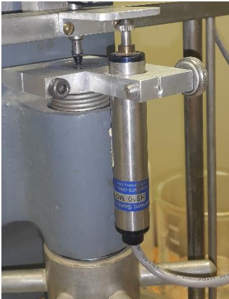
Figure 4.18: LVDT Used during Consolidation Tests
