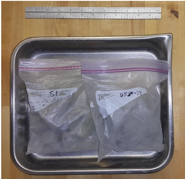
Figure 4.4: S1 and D5 Advance Glaciolacustrine Clay Samples
