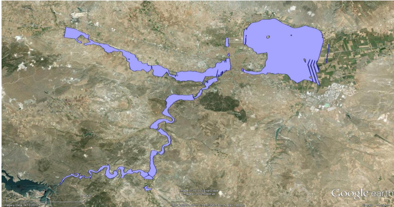
Figure 4.14. Flood Areas for Q = 300 \text{ m}^3/\text{s}
