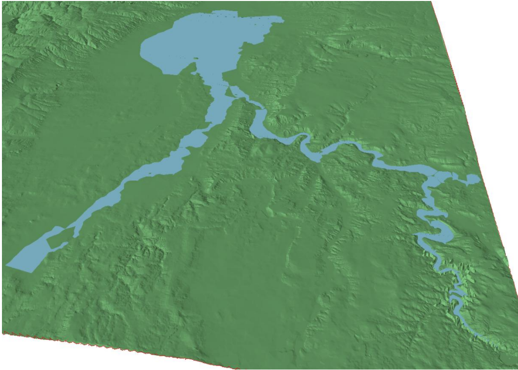
Figure 4.29. TIN and flood areas for Q = 1000 \text{ m}^3/\text{s} taken from ArcScene software
