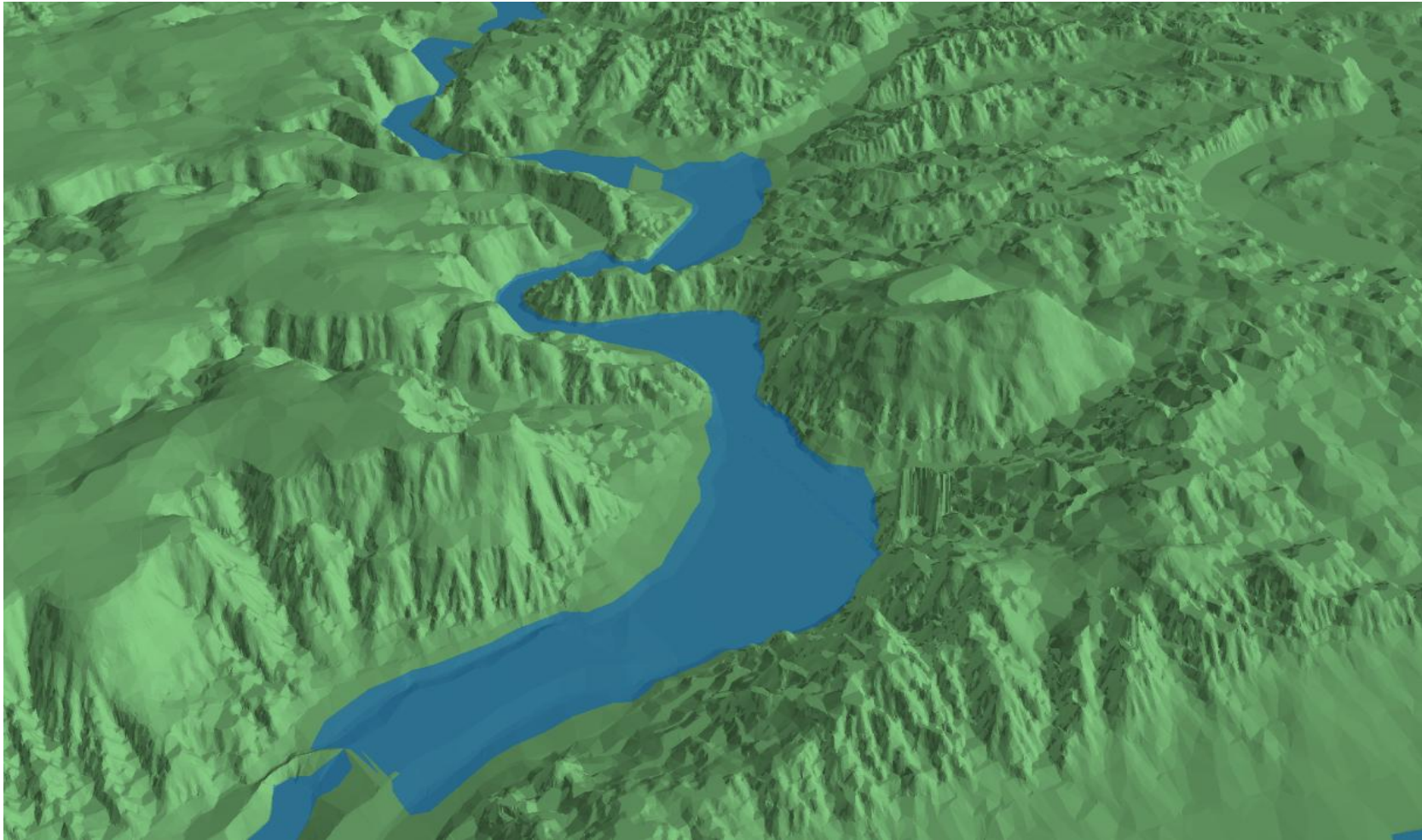
Figure 4.19. TIN and flood areas for Q = 300 \text{ m}^3/\text{s} taken from ArcScene software
