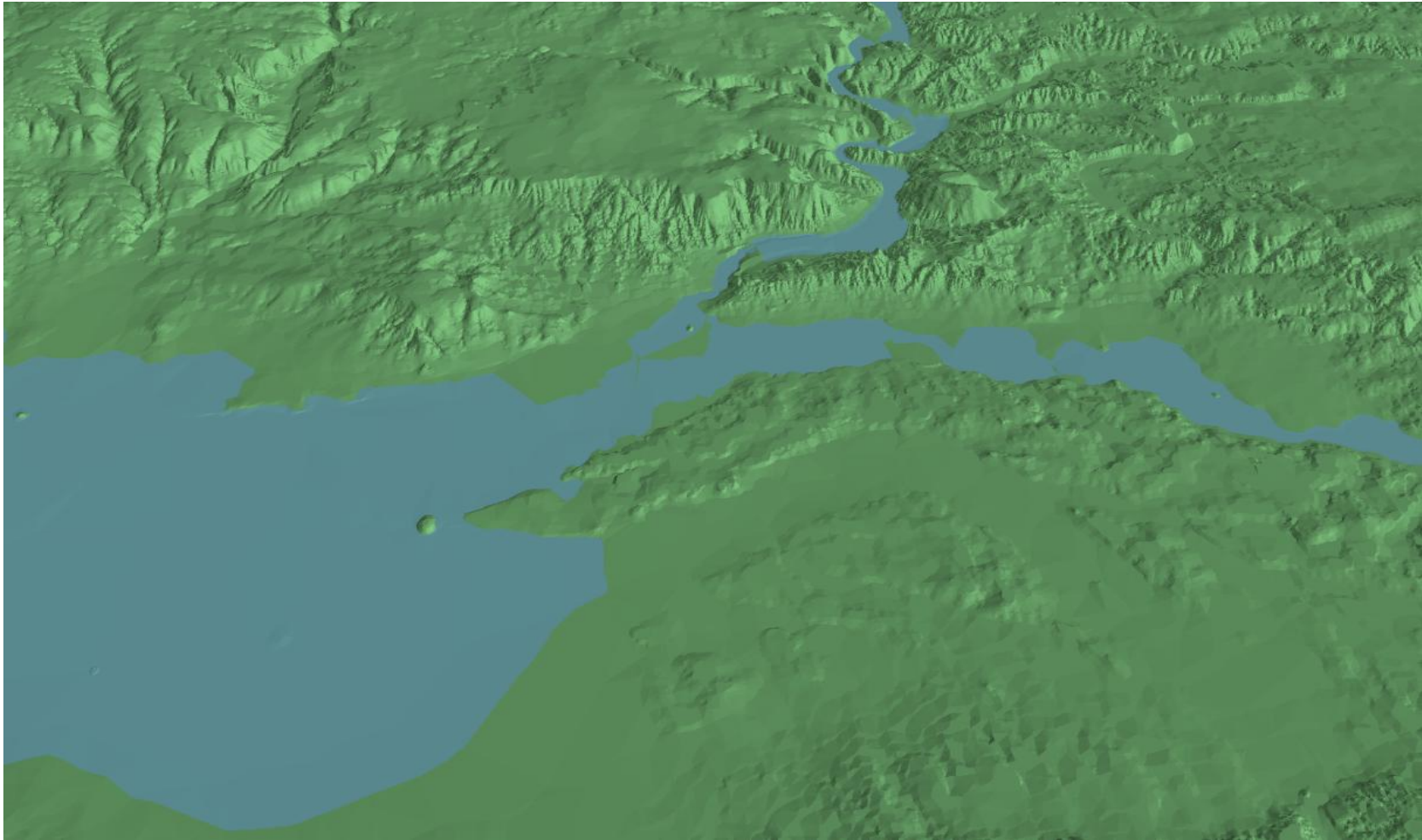
Figure 4.31. TIN and flood areas for Q = 1000 \text{ m}^3/\text{s} taken from ArcScene software
