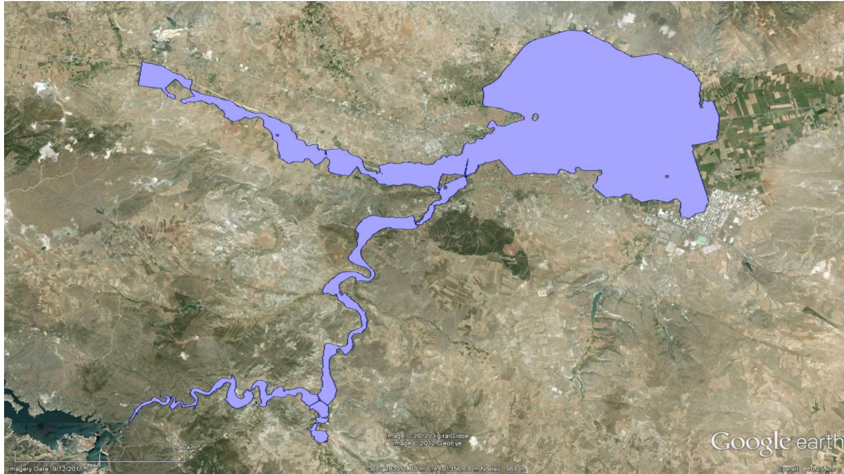
Figure 4.26. Flood Areas for Q = 1000 \text{ m}^3/\text{s}
