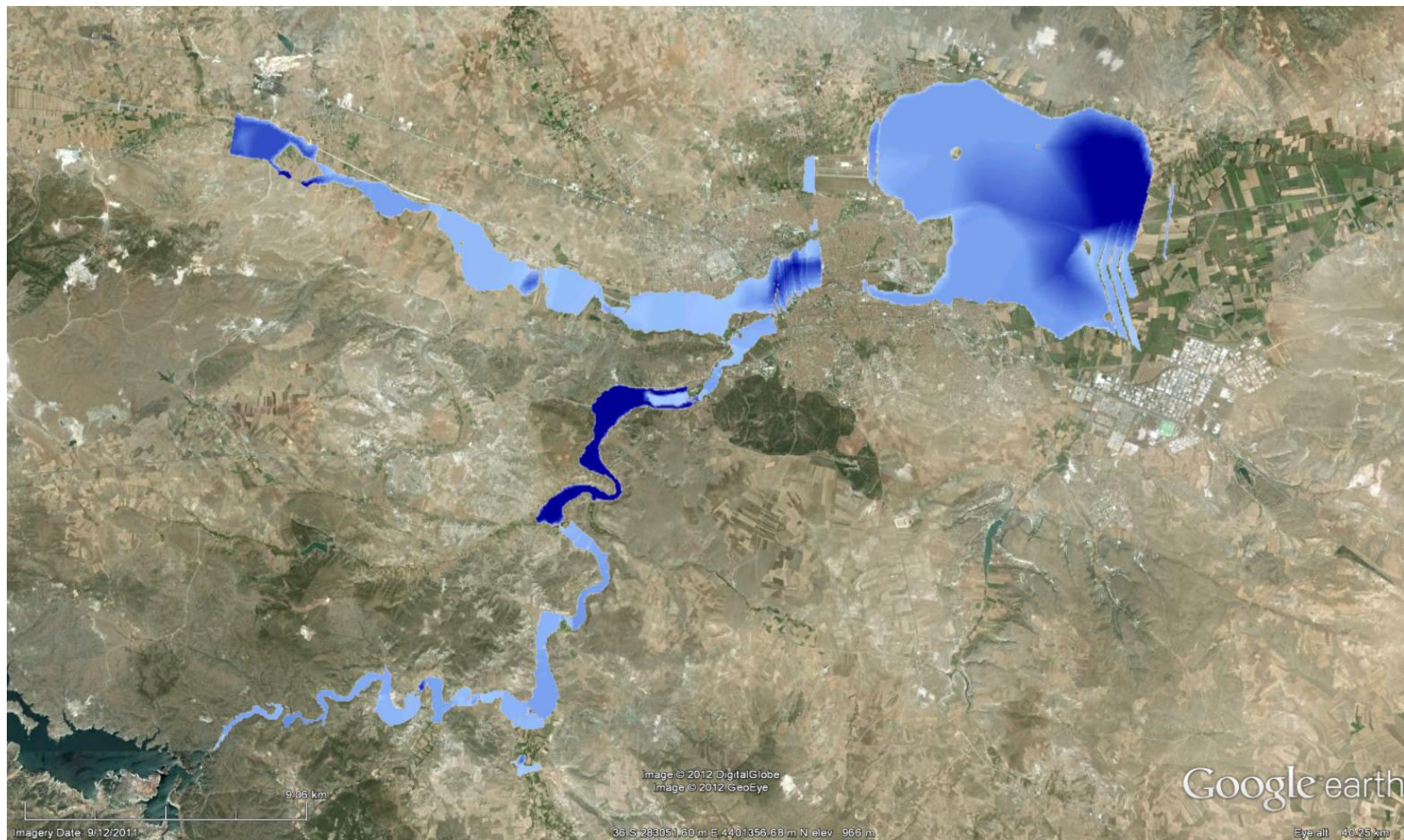
Figure 4.15. Flood Areas and Depths for Q = 300 \text{ m}^3/\text{s}
