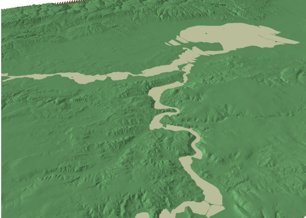
Figure 4.23. TIN and flood areas for Q = 500 \text{ m}^3/\text{s} taken from ArcScene software
