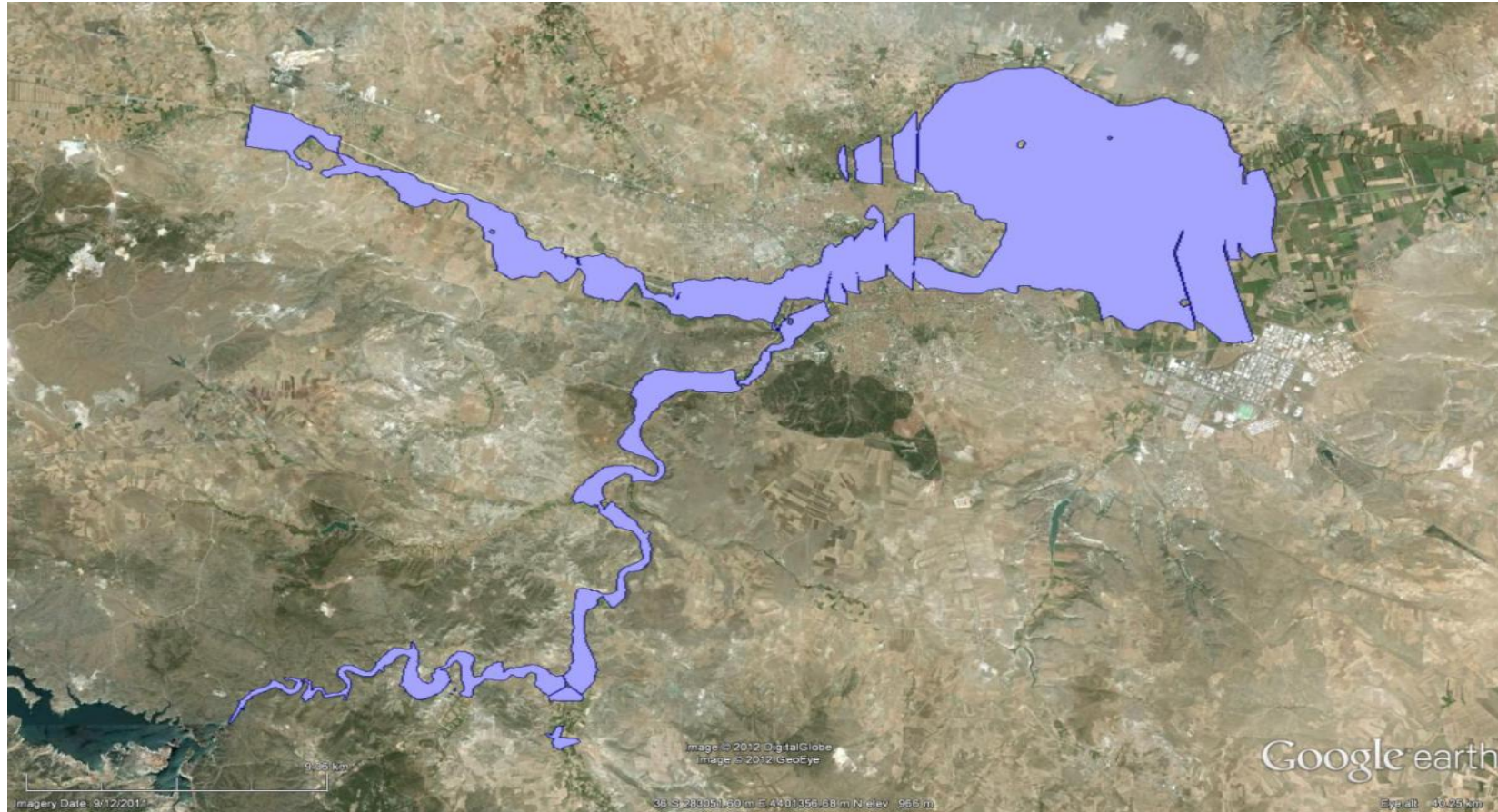
Figure 4.20. Flood Areas for Q = 500\text{ m}^3/\text{s}
